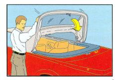
**12.** Latch the rear bow to the tonneau cover by pushing the rear bow down from its up position. Check to see that it is latched securely.
