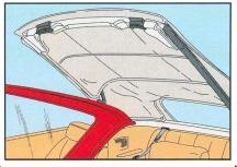
**7.** Raise the top until the front bow is against the windshield header.
