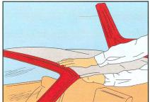
**9.** While holding the top, turn each latching handle inward and then push each handle up to its locked position.
